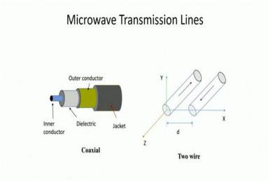
Here will consider examples of some TEM transmission lines or quasi TEM transmission lines. A very popular transmission line is a coaxial transmission line, where we have the inner conductor and an outer conductor in the form of concentric cylinders separated by a dielectric media. Another form of transmission line is a two-wire transmission line, here we have a set of parallel wires and these are used to guide electromagnetic wave from source to destination.
