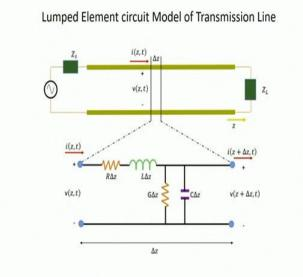
Next we show the representation of some such long elements circuit. Here we see a source is connected to a transmission line and the other end of the line is connected to the load, we considered a very small section  $\Delta Z$  of this transmission line, since the dimension of  $\Delta Z$  is now much smaller compared to the wavelength, this section can be modelled through lumped element representation. So here we have a resistance represented by  $R\Delta Z$ .
