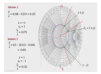
So let us now move on to how we can do this matching L section matching using a smith chart in the smith chart we first locate the point normalise impedance 2 plus j1 and then we pass a line from the centre of the smith chart through this point also we draw the constant VSWR circle and we find that as we move from the load over this VSWR circle. Towards the generator, for the first time we intersect R is equal to one circle at this point and we pass a line through this point.
