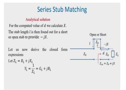
And once we have calculated the, what we can do, we calculate the value of X by substituting d, and then we find out the length of the stub so is to provide minus jX. Now let us try to see how we can derive the closed-form expression for d and l. So we have  $Z_L$  equals to RL plus j $X_L$ . We can write  $Y_L$ , which is 1 by  $Z_L$  to be equal to GL plus j $B_L$ .
