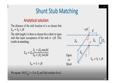
So, we start with an impedance  $Z_L$ . Now, this  $Z_L$  is to be matched to a transmission line having characteristic impedance  $Z_0$  using a shunt stub. So, first of all, what we do, we find out a distance
