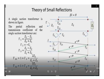
So here what we are considering, we are considering a load impedance  $Z_L$ , a transmission line of characteristic load impedance  $Z_1$  and in between we have another section of transmission line with characteristic impedance  $Z_2$  and the electrical length of this section is Beta 1 is equal to Theta. So this is essentially a single section transformer and we define the partial reflection and transmission coefficient.
