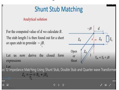
Then, once we have the computed value of d with this we find out B and then the stub length l is found for a short or open stub to provide minus jB.
