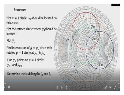
So, we follow the procedure as shown. We plot g is equal to 1 circle and YB should be located on this circle because after matching we require Yi equal to 1. Plot the rotated circle where YA should be located. Now, this rotated circle, we have seen that it is to be rotated counter clockwise by 4 pi d by Lambda.
