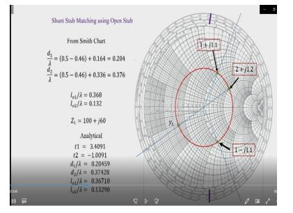
Next what we do, we verify our analytical design by comparing with Smith chart solution. So, our load impedance  $Z_L$  is 100 plus j60 which can be shown by the normalized impedance of 2 plus j12
