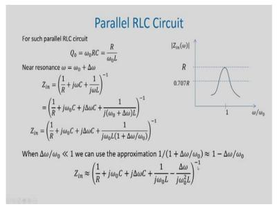
Now, Q naught the unloaded Q factor for such resonant circuit can be found out and Q naught will be equal to omega naught RC and which is also R by omega naught L. Near it is resonance the frequency angular frequency omega can be written as omega naught plus delta omega and Z<sub>in</sub> once we substitute omega is equal to omega naught plus delta omega can be expressed in this form.
