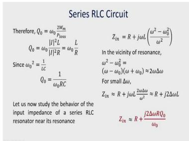
So, therefore Q naught is omega naught  $2W_m$  divided by  $P_{loss}$ , and when we substitute the term related to the energy stored in the inductor and the power loss or dissipation in the resistor then we get Q naught equal to omega naught L by R and since omega naught square is equal to 1 by LC we can also write Q naught is equal to 1 by omega naught RC we can substitute L to be equal to 1 by omega naught square C and then we will get this term.
