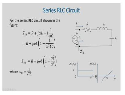
So, we consider series RLC circuit, and for the series, RLC circuit shown in the figure we can write Z in is equal to R plus j omega L minus j 1 by omega C, and then we can write  $Z_{in}$  equal to R plus j omega L into 1 minus 1 by omega square LC. Now, writing omega naught square is equal to 1 by LC. We find that Z in can be written as R plus j omega L 1 minus omega naught square divided by omega square.
