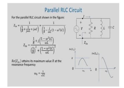
Let us now consider the properties of parallel RLC circuit near its resonance. So, the parallel RLC circuit is shown in the figure. For this type of a circuit we can write  $Z_{in}$  is equal to 1 by, 1 by R plus 1 by j omega L plus j omega C and this can be written as 1 by 1 by R minus j by omega L 1 minus omega square LC. Now, we can find out the real and imaginary parts of  $Z_{in}$  if we multiply the numerator and the denominator by the complex conjugate of this term.
