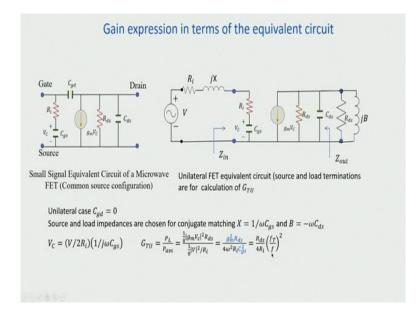
So these are the gain expressions we have seen when we consider the S parameter representation of the transistor. Now, let us look into the gain expression in terms of the equivalent circuit. In our previous module we have seen that a small signal equivalent circuit of a microwave FET, operating in common source configuration is represented like this. Now, let us consider a unilateral case. That means we assume that  $C_{gd}$  equal to 0, and also we have conjugate matching.
