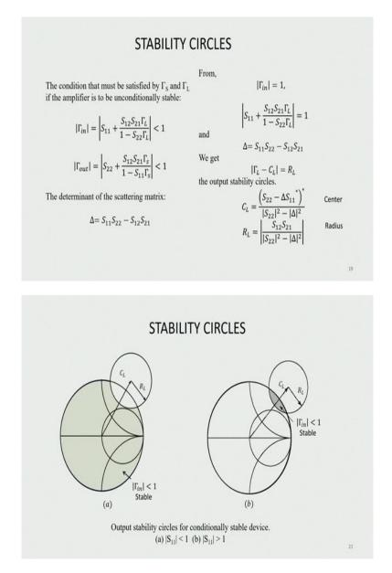
Now, from our previous discussions, we find that if the devices is unilateral. That means  $S_{12}$  is equal to 0, then mod gamma in is less than 1, if mod of  $S_{11}$  is less than 1. Similarly, mod of gamma out is less than 1, if mod of  $S_{22}$  is less than 1. So for a unilateral device, it is the values of the S parameters,  $S_{11}$ , and  $S_{22}$  that directly decides the stability.
