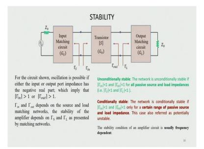
Let us now turn our attention to another very important issue in the design of the transistor amplifier circuits. This is stability. If you consider the circuit as shown above the oscillation in this circuit is possible if either input or output port impedances negative real part. So, if we have a negative real part, we can show that magnitude of gamma in will become greater than 1 or magnitude of gamma out will become greater than 1, depending on, which port impedance has negative real part.
