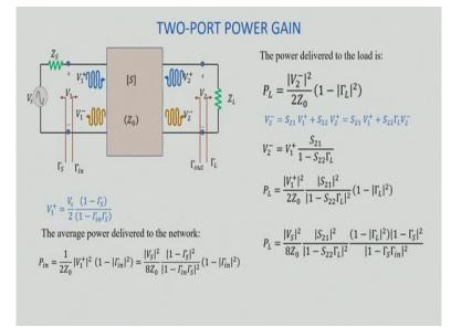
So we rewrite this expression here for  $V_1$  plus. And now, we can find out the average power that is delivered to the network P in is equal to 1 by 2Z naught, V1 plus magnitudes square into 1 minus mod gamma in square. So the incident power is mod V1 plus square divided by 2Z naught. And when this term is multiplied by magnitude of gamma in square, it gives the reflected power. And the difference of these two incident and reflected power is the input power.
