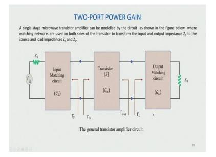
So far, we were discussing the power gain for a general two-port network. A single-stage microwave amplifier can be modelled by a circuit which is shown in the figure below, where we can see that instead of  $Z_S$  and  $R_L$ , we have Z naught as the source impedance and Z naught as the load and we have actually to matching networks, input matching network, and output matching network.
