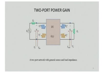
So, we start our discussion with the basics of a two-port network, and we consider the two-port power gain. This figure shows the two-port network where we have these two-port represented by its S parameter, and Z naught is the normalizing impedance of this network. We have a voltage source  $V_S$  with a source impedance  $Z_S$ , feeding the network. And also the two-port is terminated to a load impedance  $Z_L$ .
