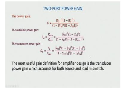
So, if we summarise our discussion, we find that we have now the expression for the power gain G, available power gain  $G_A$ , and transducer power gain  $G_T$ . Now, among these three, the most useful gain definition for amplifier design is the transducer power gain, which accounts for both source and load mismatch. Here we have both gamma S and gamma L, in the other two expressions, we get either gamma S or gamma L. And  $G_T$  has both gamma S and gamma L.
