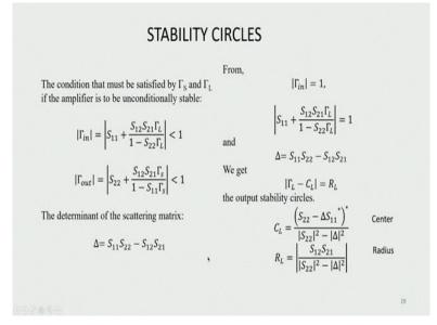
The condition that must be satisfied by gamma S and gamma L, if the amplifier is to be unconditionally stable: we have already stated mod gamma in is less than 1 and mod gamma out is less than 1. We represent the determinant of the scattering matrix S by delta, which is equal to  $S_{11} S_{22}$  minus  $S_{12} S_{21}$ . Now, if we equate mod gamma in to 1, then will get the condition that mod of  $S_{11}$  plus  $S_{12} S_{21}$  gamma L divided by 1 minus  $S_{22}$  gamma L is 1.
