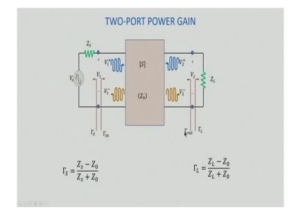
Next, we derived some of the useful relations which are necessary in order to derive the expression for these gains G,  $G_{A}$ , and  $G_{T}$ . So, we start with the two-port network. Here we can see that the reflection coefficient gamma S can be defined as  $Z_{S}$  minus Z naught divided by  $Z_{S}$  plus Z naught. As we have already mentioned that Z naught is the reference impedance, we are considering the entire system.
