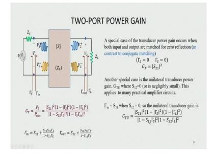
Now, let us go to some specific cases. Special case of the transducer power gain occurs when both input and output are matched for zero reflection. So, that means we have gamma S equal to 0, gamma L equal to 0. So this is in contrast to conjugate matching. Now, when gamma S and gamma L, they are 0. In that case,  $G_T$  becomes simply mod of  $S_{21}$  square.
