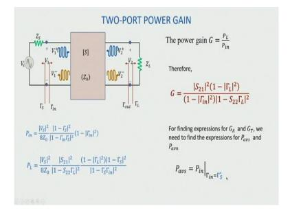
So for the two-port shown, we have  $P_{in}$  and  $P_L$  given by these expressions. And once we have these expressions, we can find out the power gain G to be equal to  $P_L$  by  $P_{in}$ . So, once we substitute the expressions for  $P_L$  and  $P_{in}$ , we get G equal to mod of  $S_{21}$  square into 1 minus mod of gamma L square divided by 1 minus mod of gamma in square into 1 minus  $S_{22}$  gamma L mod square.
