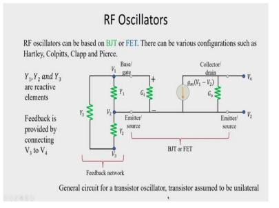
Now, the RF oscillators can be design based on BJT or FET. There can be various configurations such as Hartley, Colpitts, Clapp, and Pierce. So we will discuss a generic block diagram where this active device, this terminal can be the base, this can be collector, and it can be emitted if the device is a BJT. In case of FET this terminal is the gate terminal, this is drain terminal, and this is source terminal.
