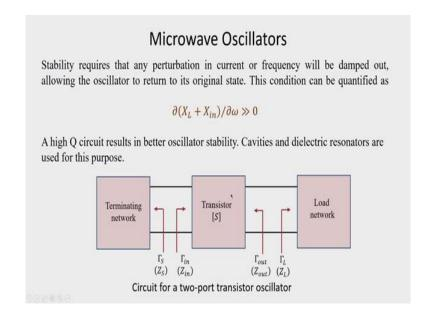
Now, stability requires that any perturbation in current or frequency will be damped out, so a small change in the current or the frequency will be damped out, allowing the oscillator to return to the original value. And this condition can be quantified as del of  $X_L$  plus  $X_{in}$  del of omega much much greater than 0. And essentially this translates into the fact that a high Q circuit results in better oscillator stability.
