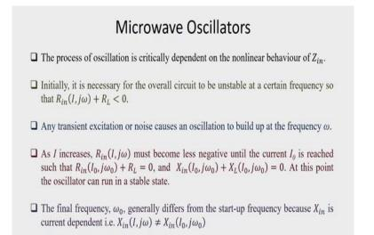
The process of oscillation is critically dependent on the nonlinear behavior of  $Z_{in}$ . Initially, it is necessary for overall circuit to be unstable at a certain frequency so that Rin as a function of I and omega plus  $R_L$ . This becomes less than 0. Any transient excitation or noise now this is how they start of oscillation is usually described. So, any transient excitation or noise causes an oscillator to build up at the frequency omega.
