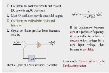
We start a new topic RF Oscillators. Oscillators are nonlinear circuits that convert DC power to an AC waveform. Most RF oscillators provide sinusoidal outputs. Oscillators are realized using diodes and transistors. Apart from diode and transistor based oscillators, crystal oscillators are also used, which provide better frequency stability.
