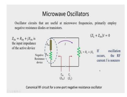
So, transistor-based oscillators what we have discussed this are useful for RF frequencies but when the frequency becomes very high, in the higher microwave frequencies, the oscillators circuits the employ negative solutions diodes and transistors. So, the devices operated in the negative resistance region, we show a generic representation where a canonical RF circuit is shown as 1 port negative resistance oscillator.
