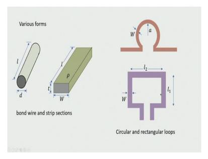
Inductors appear in various forms. So, bond wire and strip sections are shown here, and the inductance provided depends on the diameter and the length. Similarly, here the width thickness and L length. So, inductors are also realized using loops either circular loops or rectangular loops.
