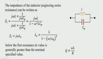
So, effective inductance is a parameter that is of importance. This is because the inductor has associated parasitic capacitance and if we represent an inductor along with its parasitic capacitance, which is represented by CP. The impedance ZI is actually the parallel combination of the reactance of L and that of CP, and it can be written as J omega L divided by 1 minus omega square LCP.
