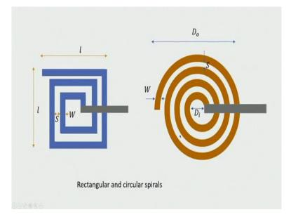
Another very popular realization of inductance is using spirals. We can have a rectangular or circular spiral as shown in the figures. And design of this type of inductors depends on determinant width, then the length, then the spacing between the individual spiral arms or determining the diameter. Again, the spacing and both analytical and numerical computations are done for finding out the dimensions of this spiral inductors for realizing specific values of
