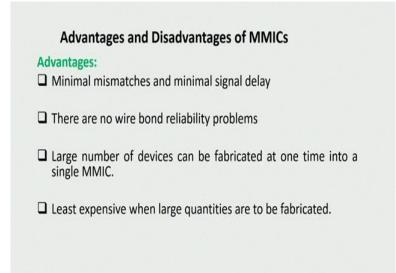
We now discuss some of the advantages and disadvantages of MMICs. The major advantages are minimal mismatches and minimal signal delay. Because everything is being fabricated on the same substrate. Wire bond reliability problems are eliminated. A large number of devices
