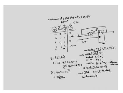
Conversion of D flip-flop into T flip-flop. So, we have to express D as a function of T. So, you take Qn, Qn+1 and you take T, this is D. This is given flip-flop you have to take at the
