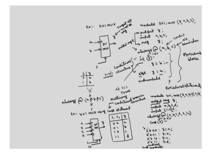
So, this is 2 by 1 MUX. You call this signal as select signal s and two inputs you call as a, b output is y. So, we know that the operation is s is 0, output should be a if I connect to 0 and this is going to 1, s is 1, output should be b. So, module 2by1MUX output is y, inputs are a, b and selection signal; output y; input a, b, s. And, because we are going to use procedural assignments so the target output must be register. So, you have to define register y.
