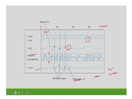
So, you can see that this is the clock, I have defined the clock as this clock is 0 and for every 5 milliseconds or nanoseconds, t clock is equal to complement of that one. This I have used in the previous example also the same logic, here also I have not given the any time scale, this can be nanoseconds or seconds ok.
