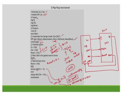
Now, how to write the test bench for this D flip flop? This is the test bench for the D flip flop. So, we will define the time scale as 1 nanosecond or 1 picosecond. So, module name we have given D flip flop tb and we know that this test bench does not have any port declarations, then the inputs will be represented by the registers. So, the inputs are D, Clock and Reset, three will be defined as registers and outputs by wires so, we have two outputs Q and Qbar, this is the first step.
