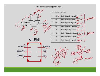
So, the next example is; so, with this introduction to this combinational sequential circuits we have written the test benches for AND gate, multiplexer and then, for D flip flop and then, zero detector. Now, I will take some case studies. So, the first case study is ALU. So, in the starting of this course itself as I have told so, after this course, you should be able to design a processor, ok. One of the main block in the processor is an arithmetic logic unit.
