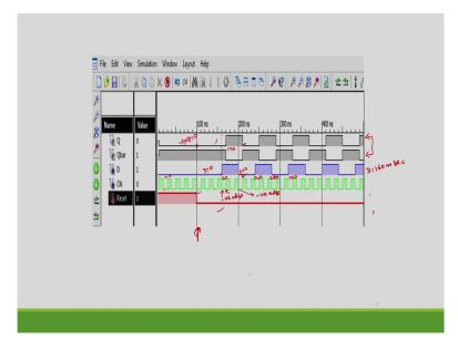
So, up to 100 nanoseconds, Reset was high, then Reset is 0. When reset is high, what will be the output? As I have told output is equal to 0 regardless of the D, Q is equal to 0 mean Qbar is equal to 1. So, these two are complements to one and the other, this is Q and Qbar. So, it is about the reset.
