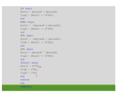
So, similar type of explanation is therefore, subtraction, multiplication, AND operation, then we have NAND operation, NOR, exclusive OR. So, finally, we will have result as initially, I will begin with by default, this result will be 0, this sets I mean both carry and zero flags will be reset.
