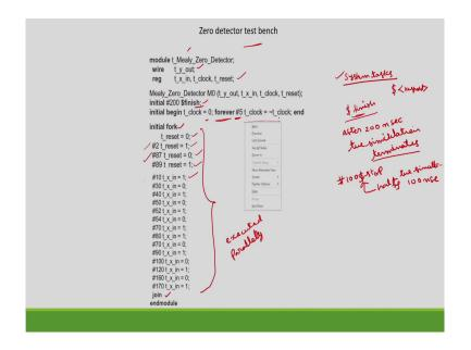
Then, we have the test bench corresponding to this. So, this is the test bench. So, here, we have taken the outputs as wire, inputs as the register as usual. Then here, you have used some extra commands like keywords like finish. So, there are some system tasks in Verilog out of which one is this. System task, the general format of the system task is dollar followed by keyword.
