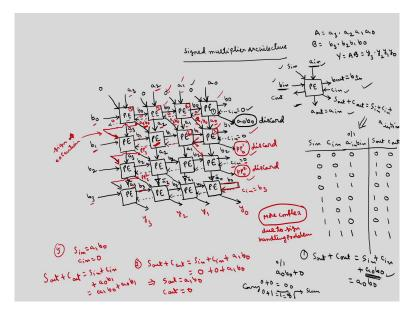
So, what is the architecture for signed multiplier? In order to map this algorithm onto architecture first we have to define a processing element. So, here I am going to define processing element as this. So, with a in is the input a out is the output and I will make a out is equal to a in.
