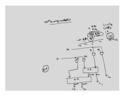
I will just start with a simple multiplication algorithm, binary multiplier. Suppose, if you want to perform 2-bit by 2-bit. So, we have A 1 A0 is one input, B 1 B 0 is another input. So, this normally, I mean conventional like conventional decimal multiplication. You have to multiply A 0 with B 0; A0 with the B 1; A 1 with B 0 A 1 with B 1.
