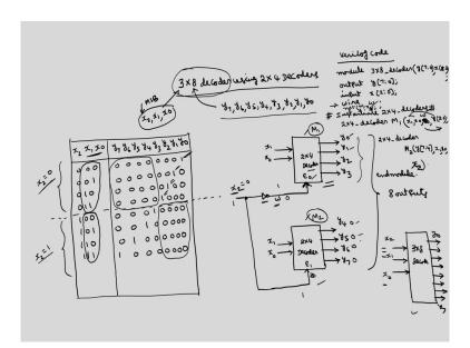
So, this 3 by 8 decoder using 2 by 4 decoders; how to construct this 3 by input 3 inputs let us call this one as  $x^2 x^1 x^0$ . This is MSB,  $x^0$  is LSB and 8 outputs you call as  $y^7$  to  $y^0$ . So, how to construct this? So, how many such 2 by 4 decoders are required? And what are the external circuitry that is required to construct a 3 by 8 decoder ok.
