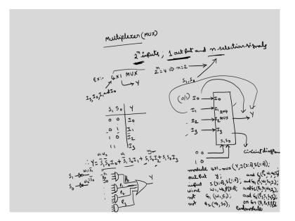
So, the next combinational circuit is multiplexer. So, this is having several applications in all the fields of electrons and communication engineering. So, this multiplexer in general will be having 2 raised to the power of n inputs 1 output and n selection lines. So, the number of inputs is normally a power of 2 the relation between the number of input and selection lines is this if n selection lines are there 2 raised to the power of n inputs, but always output is 1.
