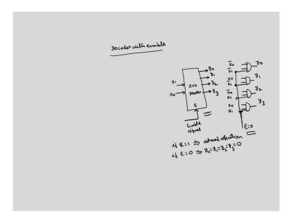
So, I will take this same 2 to 4 decoder. I am considering only positive logic for the sake of simplicity; x1 x0 I will give one more signal called enable signal E; E is enable signal. Outputs are y 0, y 1, y 2, y 3. If E is equal to 1 then normal operation; in the sense the same this truth table will be enabled this truth table will be enabled only if E is equal to 1.
