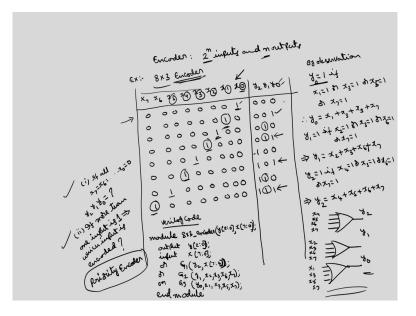
So, the next combinational circuit is the opposite of this decoder is encoder. Encoder is a combinational circuit with 2 to the power of n inputs and n outputs. This is reverse to the decoder. So, for each combination of the input, the output code will be generated which is the
