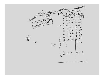
I will take a simple case of 4 to 2 priority encoder; priority encoder. A simple encoder will be having 4 inputs and 2 outputs. Here I am going to place an additional output also. So, let the inputs are x3 x2 x1 x0 with x3 is MSB x0 is LSB, outputs are y1 y0, but in addition to this y1 y0, I will include one more output.
