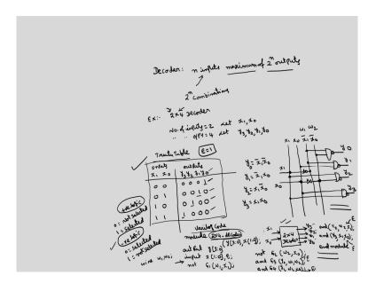
Decoder is a combinational circuit with n inputs and a maximum of 2 raised to the power of n outputs. This is maximum not always it will be equal to 2 raised to the power of n ok. For each combination of this input if we have this n inputs. So, I can have 2 raised to the power of n combinations because each input can be 0 or 1.
