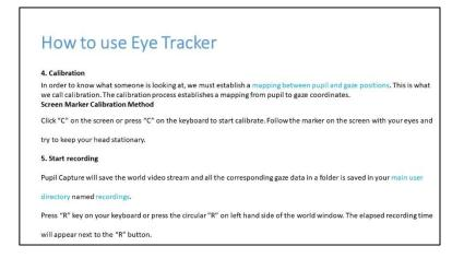
The next step is calibration - in order to know where a person is looking at, you have to calibrate your device. Calibration means it is establishing the mapping between your pupil and the gaze positions that is called as calibration.
