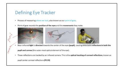
Next, let us see some of the key terminologies associated with the eye tracking device. The first one that is what mentioning is point of gaze. Point of gaze is simply if I say it is where we are looking at; at a in a particular stimuli or in real world. So, it is the process of measuring where we are looking at is called as point of gaze. The point of gaze tells you the position of your eye and the movements they make.
