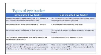
Next, let us discuss the third outline that I have told you the types of eye tracking device. So, we identified two types of eye tracking device. One is generally screen based eye tracker which is also called as remote, stationary or desktop eye tracker; and the other one is head mounted eye tracker which is also called as eye tracking glasses.
