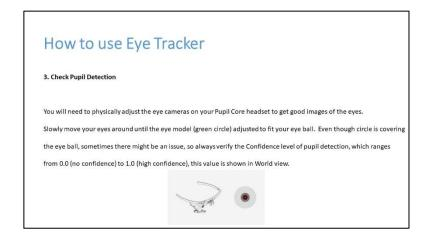
The third step is checking the pupil detection. So, you need to do it physically and adjust the camera along with your eye. And so that you can capture good images. Slowly move your eyes till the eye model that is a green circle adjusted fit your eyeballs even though if you are getting the green circle ensure the confidence. Confidence by which your eye gets captured.
