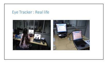
Next these are some of the images that we captured during an experiment in a laboratory using eye tracking devices. Now, as I said there are various types of eye tracking devices. This is a stationery or a remote or desktop eye tracking device which is usually located at the bottom of a screen.
