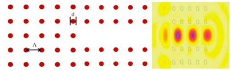
Figure 1: Photonic crystal structure. (Left) The diameter of the dielectric column is d and the spacing between the dielectric columns is the lattice constant \Lambda . (Middle) PBG structure. (Right) PBG light guiding
