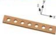
Figure 2: Example of a periodic dielectric waveguide, which combines one-dimensional periodicity (in x ) and index-guiding in two transverse directions.
