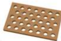
Figure: Examples of photonic-crystal slabs: The hole slab , a triangular lattice of air holes in a dielectric slab.
