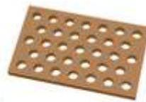
Figure: Examples of photonic-crystal slabs: The hole slab , a triangular lattice of air holes in a dielectric slab.
