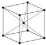
BCC Conventional Unit Cell
