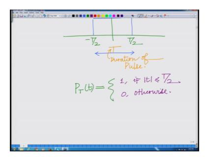
So, this is the width of the pulse or duration of pulse this is the duration of the pulse; pulse is from minus T by 2 to T by 2 this is denoted by p sub capital T of t where P sub capital T of t equals well this is equal to one if mod t less than or equal to capital T over 2 0 0 otherwise. So, this is or pulse now what we are going to do with this pulse if have to illustrated in a very simple fashion the first symbol let us say this is my time access.
