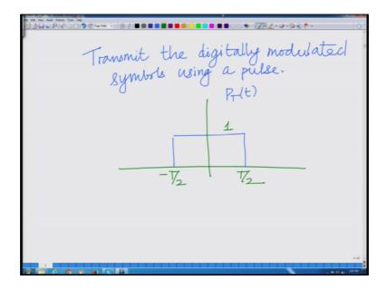
So, this particular signal is termed as a pulse how do you transmit the digital modulated symbols. So, we transmit the digitally modulated symbols using a pulse for instance a typical pulse a typical pulse can be of the form. So, this is let us say a pulse P T we are already seen an example of the pulse one of the previous modules pulse can be of height 1 from minus T by 2 to T by 2. So, capital T is the width of the pulse.
