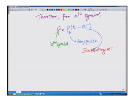
So, what we are absorbing is basically it is very simple it is therefore, for kth symbol you have a k the pulse P I am just calling it P T minus k T, their P is any pulse not necessarily P subscript T capital T. So, this is any pulse shifted by k T where T is the symbol duration and a k is a kth symbol.
