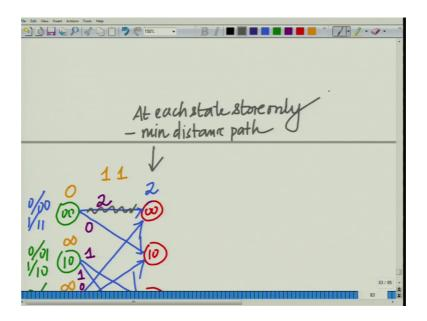
So, to 00 at time instance j equal to 1 the minimum distance is 2 and minimum distance path is from 00 take the top branch with output 00 and branch metric 2.
