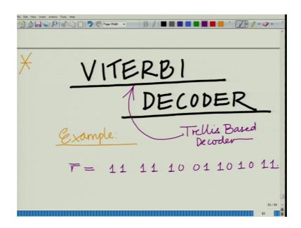
So, what we are going to look at is the Viterbi decoder for a convolutional code, which was proposed by an Viterbi. And we are going to illustrate this trough an example. So, we are going to consider an example. And of course, was without saying this is a trellis base decoder that is by we have been building up and emphasizing the importance of the
