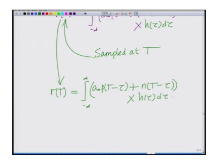
So, sample at T which means I have to substitute small t equal to capital T that is nothing but minus infinity to infinity a naught P of capital T minus tau plus n of capital T minus tau times h of tau d tau this is the output signal r t output of the linear time invariant system r t sampled at capital T, where capital T is the symbol duration.
