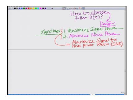
So, that is something that is fundamental which you might already seen before. So, the objective is. So, we have dual objectives really cycle call object. So, objective is maximize signal power 2 to minimize the noise power. So, I would like to maximize and both these things together you would like to maximize signal to noise power ratio this is defined as SNR. So, this is a fundamental quantity in the analysis of communication system.
