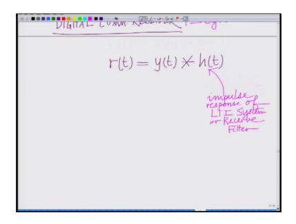
That is output when y t is passed through h t that is r of t, I can say r of t r of small t that is a continuous time signal is y t passed through h t when it when you pass a signal through a linear time invariant system correct the output is the convolution of the signal with the impulse response. So, h t is basically nothing but the impulse response of the LTI system or the impulse response of the receive filter.
