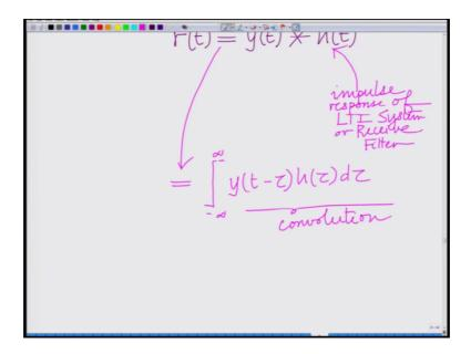
Now therefore, I can write this remember the convolution can be expressed as the integral minus infinity to infinity y, t minus tau h of tau this is the convolution operation continuous time convolution or infect linear convolution and now we know let us assume we know the transmitted we know well what do we know.
