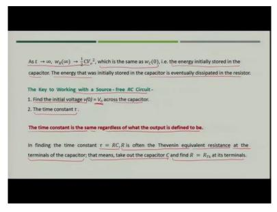
Now if you see this equation at time t is equal to 0, the energy will be 0. When say that at time t is equal to infinity the term in the bracket will become 0, so.
