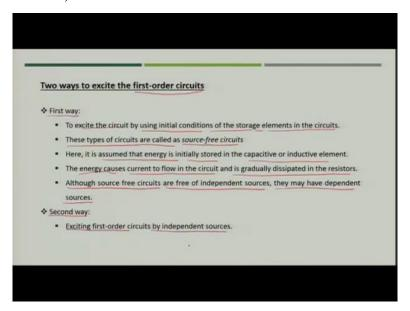
Now we have two ways to excite these first order circuits. The first way is by using initial conditions of the storage elements in the circuit, so that means that initially if you charge either capacitor or inductor and insert that charged capacitor and the inductor into the circuit then, the circuit will have only the source of energy as the total energy stored in either capacitor or inductor.
