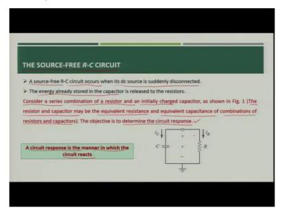
First let us try to understand what you mean by source free RC circuit. Source free RC circuit means we do not have any external voltage or currents source connected to the circuit.
