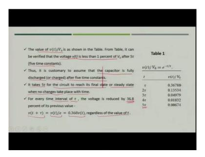
So, if you plot the value of  $v(t)/V_0$ , that is, if you take  $V_0$  in denominator so, this will become  $v(t)/V_0 = e^{-t/\tau}$ . We will plot this value with respect to time t and let us take time t as a multiple
