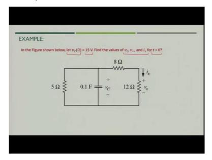
So, let us now, understand the concept with the help of one example so that you can understand the concept clearly, if you see this particular figure in this figure let the initial voltage across capacitor is, 15 volts so, what we have to do, we have to find the value of  $v_C$ ,  $v_x$ ,  $i_x$ .
