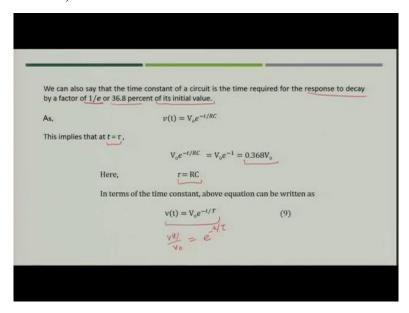
Now, what does it mean let see, so when we say that the time t is equal to time constant the response will decay by a factor of 1/e that is e to the power minus 1. It means that it will decay by 36.8 percent of its initial value. When we simplify by replacing RC as t is equal to  $\tau$ , we get this value, so we say that when we represent  $\tau$  in the circuit,
