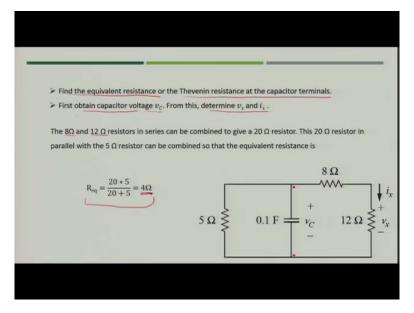
So, what you will do, first we will find the equivalent resistance or you can say the Thevenin resistance at the capacitor terminal, and then we will obtain the capacitor voltage and then, from  $v_C$  we will determine the value of  $v_x$  and  $i_x$ . Now, 8 ohm and 12 ohm resistors are in series and this combination is in parallel with 5 ohm resistance. From the calculations in the above slide it can be seen that R equivalent is 4 ohms.
