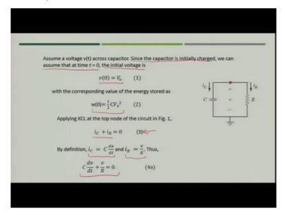
Let see how the performance of the circuit would be when you have the capacitor initially charged and connected to the resistor in parallel. in this case since, capacitor is initially charged so, we can assume that suppose time t is equal to 0, the capacitor was having some initial voltage say,  $V_0$ . This initial voltage is the voltage across the capacitor at time t is equal to 0.
