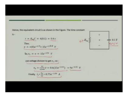
So now, finally the R equivalent that is 4 ohms, is connected in parallel with 0.1 Fared capacitor who is having initial voltage as 15 volts. From the above slide, the calculations can be seen to find the unknown parameters.
