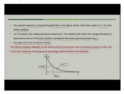
Now, how you will represent it graphically when you represent the natural response graphically it will be, like as shown in the figure, below, so here you will see when you have the component  $v(t) = V_0 e^{-t/RC}$ . Let us assume that the there is another component called time constant and it is denoted by Greek letter  $\tau$ . Let us say that this time constant  $\tau = RC$ . Therefore,
