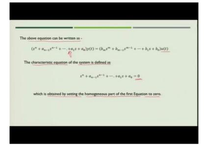
Now, if you are given the transfer function, how to find the characteristic equation? Now, let us consider the system given by the differential equation same differential equation we are using which we saw in the previous case. Now, the Laplace transform of this we saw equal to this. Now, what is y(t)/u(t)? This is nothing but the transfer function of the system, so
