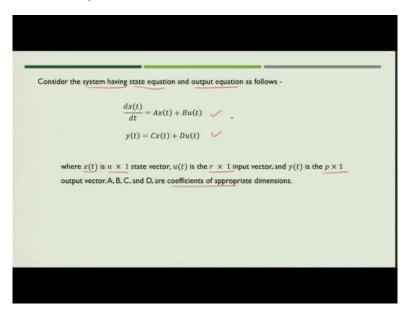
Now, let us consider the system, we have state equation and output equation that is the standard state and output equation given as follows that is
