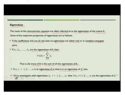
Now, let us try to understand what eigenvalues is. So, the roots of the characteristic equation which we just discuss are refer to as the eigenvalues of the matrix A. So, what are the important properties of eigenvalues? So, if the coefficients of A are all real then its eigenvalues would be either real or in complex conjugate pairs.
