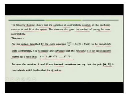
Now, the following theorem shows that the condition of controllability depends on the coefficient matrices A and B of the system. And we are particularly talking about the state controllability that is why A and B Matrices are being considered for the controllability analysis. Now, theorem also gives the method of testing for the state controllability. What is the theorem? Theorem says that for the system described by the state equation that is  $\frac{dx(t)}{dt} = Ax(t) + Bu(t)$ .
