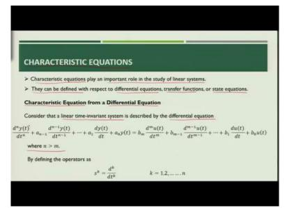
Now, if you put that into the above equation, so the above the differential equation and what we have saw, recently we can write in terms of Laplace transforms. So, what we can write? Instead of writing the differential equation it can be expressed as,
