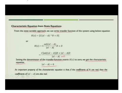
Now the third case, when you need to find out the characteristic equation from State equation. So, when you, we were discussing about the State variable approach we found that the relationship between State variable coefficient matrices and the transfer function is as follows. So, the transfer function from the State variable we can get  $H(s) = [C(sI - A)^{-1}B + D]$ .
