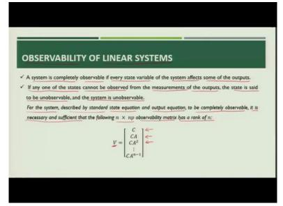
Now, let us understand with the help of the example. So, the condition that is containing A and C both matrices, we generally call it as the pair that is [A, C] is also observable.
