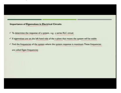
Now, what is the importance of eigenvalues? These eigenvalues help in determining the response of the system say if you have a series analyses circuit. So, if you converted into State variable firm and find the eigenvalues these eigenvalues will help us in finding out the response of the system. If the eigenvalues are on the left inside of the splane that means if they have the real component negative. That means that the system is stable.
