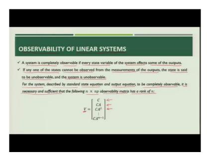
Now, let us understand another concept called observability of the linear system. Now, the system is completely observable if every state variable of the system affects some of the outputs. That means that if anyone of the states cannot be observed from the measurements that is the output measurements, the state is said to be unobservable and therefore the system will be unobservable.
