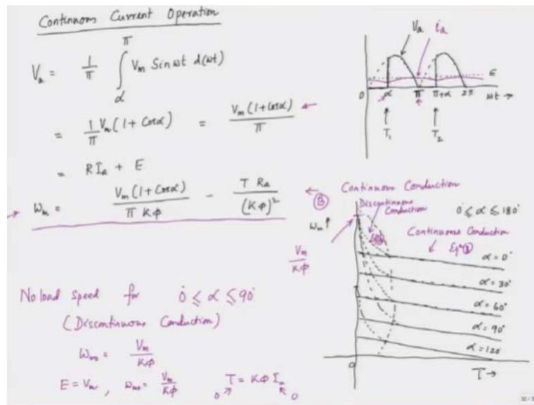
In continuous conduction mode, there is typically some back EMF, denoted as  $E$ . Here, we note that the speed is relatively low, resulting in a lower back EMF. The current waveform in this mode does not drop to zero; instead, it begins from a certain value and maintains a continuous flow throughout its cycle. This characteristic shape illustrates that the current never reaches zero.
