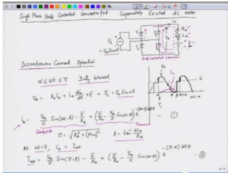
Now, let's take a closer look at the circuit diagram of a half-controlled converter. In this configuration, we have two Silicon Controlled Rectifiers (SCRs) and a diode, which supply power to the armature of a DC machine, specifically a separately excited DC motor. The armature consists of resistance, inductance, and the back electromotive force (EMF), denoted as E.
