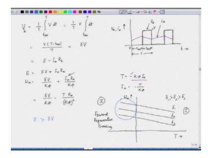
Now, let's take a closer look at the waveforms of the voltage and current for the circuit we just discussed. During the energy storage interval, which lasts from 0 to  $t_{ON}$ , the voltage across the armature is zero. Therefore, when we plot the armature voltage,  $V_a$ , on the y-axis against time on the x-axis, we observe that the armature voltage remains at zero while the current builds up.
