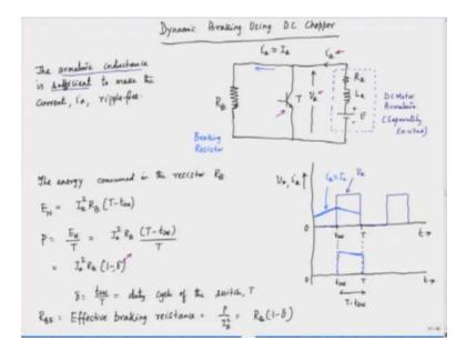
What we have here is the armature of the motor, which is represented by its resistance, inductance, and back EMF. Connected in parallel with the armature is a chopper switch, which interfaces with a braking resistor, denoted as  $R_B$ . This chopper switch is represented by the transistor T. We can define the armature voltage as  $V_a$  and the armature current as  $I_a$ .
