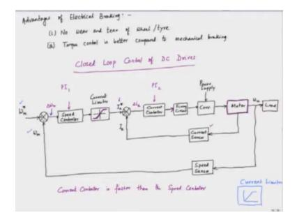
The advantages of electrical braking, whether through regenerative braking, plugging, or dynamic braking, are numerous. First and foremost, there is no wear and tear on the wheels or tires because the motion of the wheels is halted electrically. This means there is no friction between the wheel and the road or railway track, which significantly extends the life of these components.
