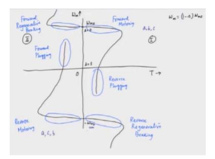
If we were to illustrate the torque-slip or torque-speed characteristics, we can plot the data derived from Equation 1 to create a visual representation. On the X-axis, we will have the torque, while on the Y-axis, we will depict the speed. It's essential to note that the speed and slip are related through the equation  $\omega_m = (1 - s) \omega_{ms}$ . This relationship means that as slip changes, so does the speed.
