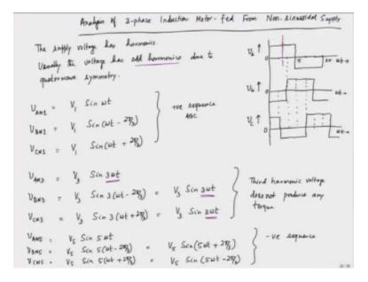
Let's delve into the analysis of a three-phase induction motor powered by a non-sinusoidal supply, specifically one that contains harmonics. In this scenario, if we use an inverter to supply the motor, we may observe that the waveforms for phases A, B, and C are not sinusoidal. For instance, consider the voltage for phase A; instead of a smooth sine wave, it manifests as a square wave.
