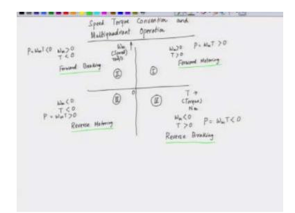
Now, let's delve into the speed-torque convention and the multi-quadrant operation of electric drives. We have established that in electric drives, two key mechanical variables come into play: speed and torque. It is essential to control both the speed and torque of the motor, as these outputs are critical to the motor's performance.
