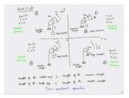
Quadrant 4 is characterized as reverse braking. Now, let's delve into a practical example of this four-quadrant operation. Consider a hoist, which can simply be referred to as a lift that transports either a person or materials. In examining the hoist, we aim to understand its operation across the four different quadrants.
