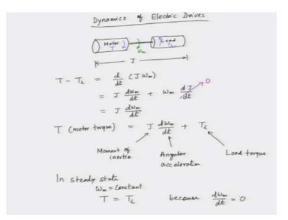
Now, let's explore the relationship between speed and torque in our system. We have a motor that is mechanically coupled to a load, and we need to examine how these components interact. In this setup, the motor produces a torque T in one direction, while the load generates an opposing torque, denoted as T<sub>1</sub>. This load torque resists the motion of the motor.
