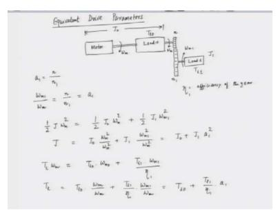
Now, this motor-load combination is connected to another system via mechanical gears. In this setup, we have Load 1, which is driven by the motor through a gear mechanism. The gear on the motor side has n teeth, while the gear on the load side has n<sub>1</sub> teeth. Consequently, the motor speed  $\omega_m$  drives the load at a different speed, denoted as  $\omega_{m1}$ . This discrepancy arises because the gear ratio is not equal to 1.
