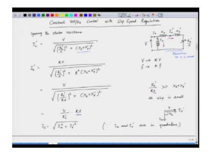
In this discussion, we will focus on constant volt/hertz control combined with slip speed regulation, allowing us to effectively manage the slip speed. Let's start by writing the equation for the rotor current. The rotor current, denoted as I<sub>r</sub>, can be expressed as the applied voltage divided by the square root of the sum of the squared rotor resistance divided by slip and the squared sum of the stator reactance and rotor leakage reactance. Mathematically, this is represented as:
