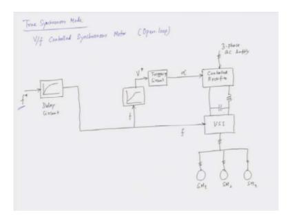
On the other hand, in the self-controlled mode, the frequency is controlled as a function of the rotor speed. This means that the stator frequency is influenced by rotor position feedback. Typically, the drives operating in true synchronous mode are open-loop systems, lacking position feedback. In contrast, self-controlled mode drives operate as closed-loop systems, incorporating feedback mechanisms to enhance control and performance.
