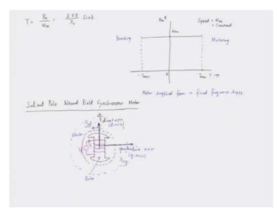
In this discussion, we are focusing on the two synchronous reactances present in the salient pole synchronous motor. We have the direct axis, denoted as  $X_{sd}$ , and the quadrature axis, represented as  $X_{sq}$ . To accurately illustrate this, we need to draw the phasor diagram for the salient pole synchronous motor.
