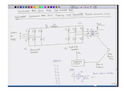
The input to the source-side converter is a three-phase AC supply, which we can label as phase A', phase B', and phase C'. Within the DC link, the large inductor ensures that the DC link current remains nearly constant and free from ripples, allowing for smooth operation.
