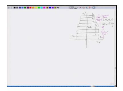
Let's take a moment to examine the torque-speed characteristics in the True Synchronous Mode. In this scenario, we are varying the frequency, which is depicted on the x-axis as torque and the y-axis as speed. Here, we see that these are constant speed drives, with a maximum torque  $T_{max}$  and a corresponding negative maximum torque  $-T_{max}$ .
