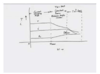
Initially,  $\theta_0$  is kept constant while we operate in chop mode, which is specifically known as current chopping mode. As we progress, we gradually increase  $\theta_0$  to maintain that constant current. What we observe here is that the current I remains steady, which in turn allows the product  $T \cdot \omega$  to also stay constant. The power can be expressed as proportional to  $\theta_0^2$ .
