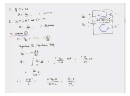
In our switching circuit, we can visualize the winding inductance as follows: our goal is for the current to be present only during the intervals of positive  $\frac{dL}{d\theta}$ . When switch T is turned on, current begins to flow through the circuit, resulting in a positive voltage across the winding, specifically,  $V = +V_{dc}$ . However, when switch T is turned off, the diode conducts, allowing the current to continue flowing in this direction.
