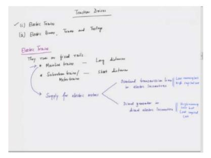
Our next discussion will focus on traction drives. When we refer to traction drives, we primarily mean electric trains, which represent one significant category. Additionally, we include electric buses, trams, and trolleys in this classification. Electric trains are designed for higher power applications, typically operating in the megawatt range, with a typical rating of around 6,000 horsepower or even more.
