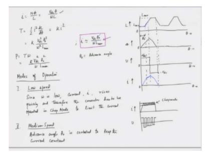
Let's examine how we switch the various voltages in our system. When we plot the variation of inductance against the rotor angle  $\theta$ , we find that the graph resembles a trapezoidal signal. This inductance starts at zero, and our objective is to ensure that the current only exists during the rising phase of this inductance.
