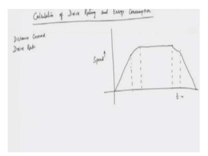
To determine the distance covered by the locomotive, we must look at the area under the speed-
