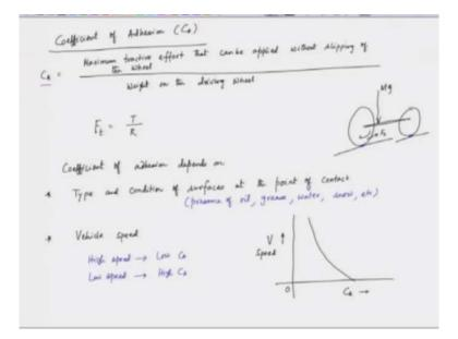
The coefficient of adhesion, often denoted as CA, is a critical parameter in understanding the traction of wheels on a track. So, what exactly does this coefficient represent? Simply put, the coefficient of adhesion is defined as the maximum tractive effort that can be applied without the wheels slipping, divided by the weight resting on the driving wheels.
