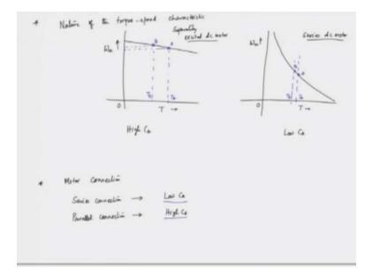
When the vehicle speed is low, the coefficient of adhesion is high, illustrating a direct relationship between these two factors. However, the coefficient of adhesion also depends on other parameters, such as the nature of the torque-speed characteristic of the motor being used.
