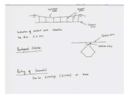
Let's discuss how power is supplied to electric locomotives. Above the train, we have catenary cables, which form the essential catenary line. Alongside this, there is a contact wire with which the locomotive establishes contact. This contact wire is maintained almost horizontally by what we call dropper wires. These dropper wires provide crucial support, ensuring that the contact wire remains nearly horizontal throughout its length.
