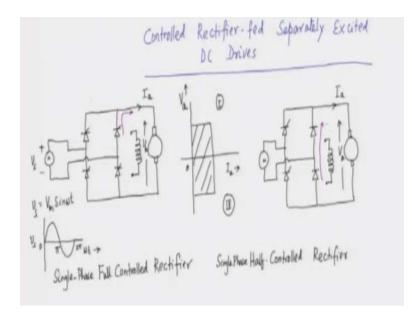
Now, let's explore the different types of controlled rectifiers we have. Primarily, there are two types: the full-controlled rectifier and the half-controlled rectifier. Let's start by looking at the topology of these two rectifiers.
