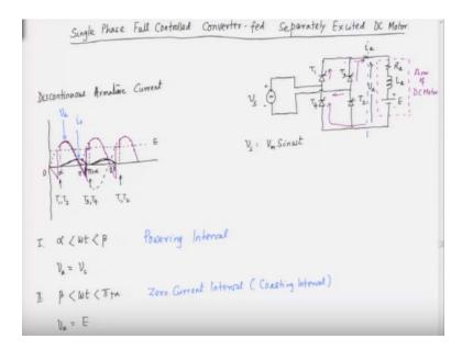
We are feeding a separately excited DC motor from a single-phase full-controlled converter. Let's begin by drawing the circuit diagram to visualize the setup. We have a single-phase bridge with four SCRs, and to simplify the motor's representation, we replace it with its equivalent circuit. This equivalent circuit of the motor includes the armature, which consists of resistance, inductance, and a back EMF.
