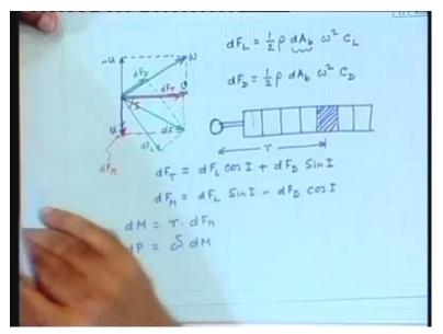
So, in order to calculate all these, we will need to use v, right, we cannot use that velocity. So, what is this v? It is the velocity of the wind as it passes over the blade. How much should it be? Yes, right, right. We have seen earlier when we were, we were calculating the maximum possible efficiency that is achievable, we found that that is attained at, yeah, beta is not necessary now. It is clear that the speed should be two third of the v infinity; that is what we have.
