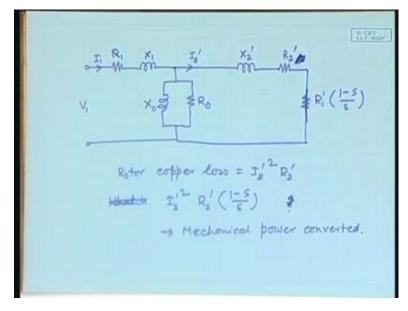
So, this is, this is the mechanical power, right. The moment you have the mechanical power it is trivial to obtain the torque. Why? Because the mechanical power is the torque times the angular speed.
