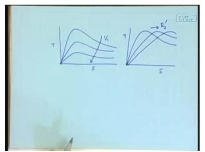
Just to drive the point home, if you vary the input voltage it will go from here to here to here. So, V 1 is being pushed down, slip versus torque and if you vary the rotor resistance, then it goes like this, clear. That is about all that we need to know from the motor side in order to go into the generator side. So, now we will discuss the generator.
