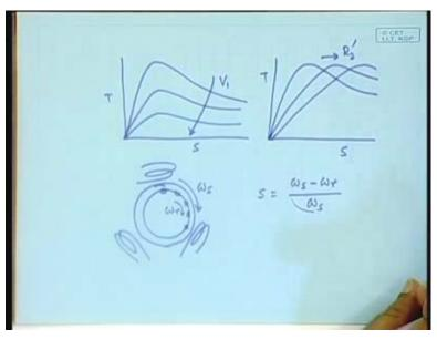
If you have the stator like this, the stator has windings like this which I drew schematically and I said that the stator field rotates with the speed omega S and there is a rotor which has conductors and the conductor fellows are rotating at omega r and so far we said that the slip is omega S minus omega R by ... Now, you had energized the stator
