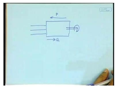
So, one important thing to remember is that if you, if you consider the induction machine as a black box connected to a three phase line and here is a shaft that is being rotated, then you have to, it is important to remember that the active power flows likes this and the reactive power flows like that. This is unique to the induction machine, induction generator, clear.
