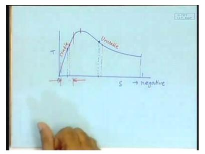
Obviously you will not make a bad machine, you will make a good machine and since if you make a good with a good efficiency, it has a very narrow range of available speed. Only this much, this much variation will be allowed and in fact, in very good machine this is even more steeper which means very little scope of speed variation.
