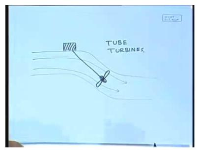
One is where the channel is not exactly vertical but it is something like this and the turbine is situated here and the shaft goes like this and the turbine is situated here. Obviously, that will allow the use of a larger, of a smaller head. These are called the tube turbines. So, there the head is smaller than the vertical axis turbine. So, this can work in lesser head.
