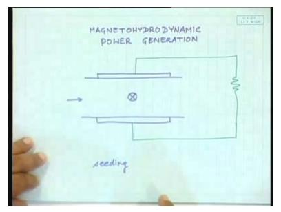
Remember, we had initially considered that this will be the direction of flow, so the electrons will be flowing like this and you have produced a B, due to which there will be a voltage generated here. That means the electrons will be actually moving like this. That is producing what is the, what you know as the Faraday effect. So, let us quantify this Faraday effect.
