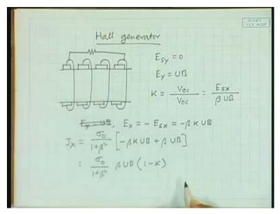
That is called the Hall generator. It is not difficult to figure out the structure of the Hall generator, because here there will be this channel and there would be the separate electrodes, remember. But now, you are trying to utilize the Hall effect which is in the x
