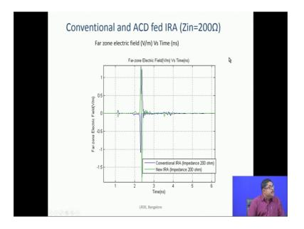
And this is the electric field how it looks like for a given very nanosecond type of a thing. Then this is the gain. So, the ACD feed that is better compared to a slightly better.
