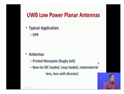
Now low power. UWB you see one typical application of low power things are making ground penetrating radar which all the applications I have said about this except communication. They can be done. So, various options are there are printed monopoles rugby ball antenna, then there were Vivaldi antennas, there were bow-tie antennas etcetera.
