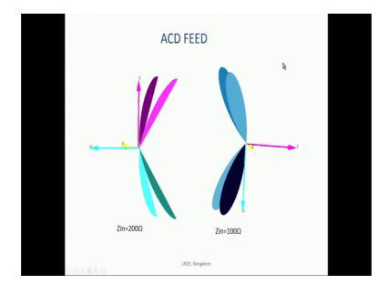
And finally, ACD Asymptotic Conical Dipole feed this is the thing.
