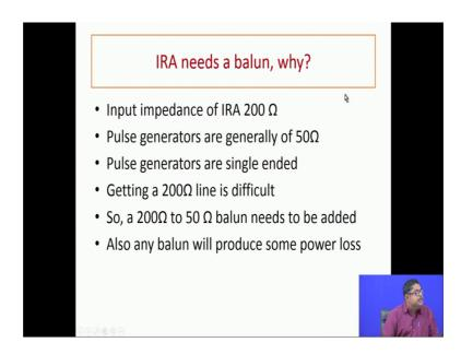
Now, IRA basically needs a balun typically, because the conventional IRA that was designed that has an impedance of 200 Ohm. Now, pulse generators generally you know electronics industry produces generators with 50 Ohm. So, also pulse generators are single ended. So, getting a 200 ohm line is difficult. So, a 200 ohm to 50 Ohm balun
