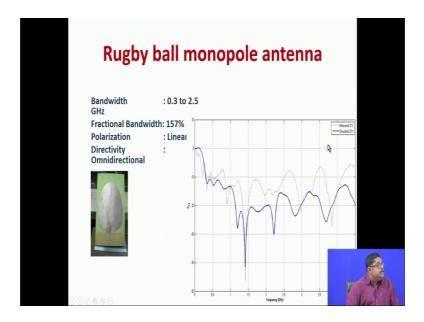
Now, let us say one of the antenna rugby ball monopole antenna. Its bandwidth you see 0.3 Gigahertz to 2.5 Gigahertz. And fractional bandwidth from that definition, if we calculate it gives 157 percent bandwidth. Its polarization is linear, directivity is omnidirectional. This is the impedance bandwidth you see from 0.3 to 0.25 it is working.
