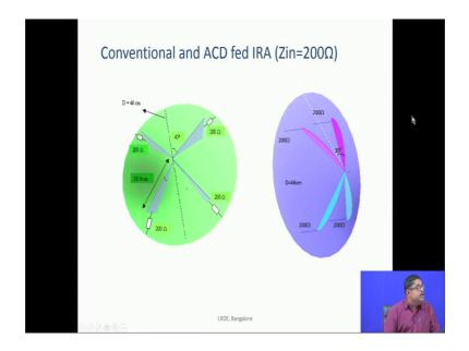
So, actually conventional IRA was designed from coplanar plates, but it was found out that it has an input impedance of 200 Ohm. So, ACD also can give you that, but the beauty of asymptotic conical dipole is that it can be amenable. So, you can make IRA with any input impedance. So, here it is showing that 200 Ohm.
