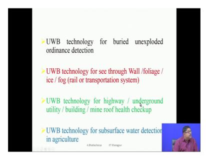
But, more than communication actually this technology has so many other applications. So, UWB technology particularly in the form of radars which are a different kind of radars than the conventional radars. So, UWB technology can be utilized for seeing whether there is any buried unexploded ordinance. Actually, in an what tone country there are many mindset sector are kept. Also sometimes many arms ammunitions some ieds etcetera they are kept.
