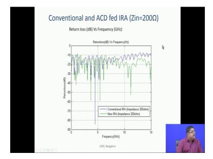
But, this is the comparison. And it can be proved that these ACD feed things that gives a better gain also. This is a return loss you see typically 10 dB is the impedance bandwidth.
