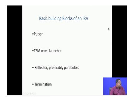
So, basic building blocks of an IRA, one is a pulser that they call that pulse source it is a high power pulse. So, then there is a TEM wave launcher. Then there is a reflector you can have any type of reflector, but preferably paraboloids are used and then some terminations.
