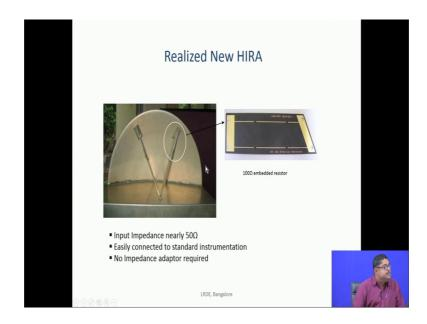
This is a the half HIRA. This is it is input impedance. So, you see 100 to 50 Ohm it is varying. Certain times it is going even below 50 Ohm, but this is good with the thing. And this is the excitation. If you give an excitation of this, this is the measured voltage at a distance. So, you see that faithful it is reproducing this. There is no dispersion here. And this is the impulse response of the HIRA.
