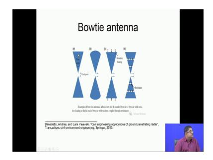
Another option is bowtie antenna. Actually this type of this is a dipole from that actually people have modified this. And then put some resistive loading to cut off various high frequency undesired things. Then there are instead of loading at the lamp once people have also loaded here. So, this is one in civil engineering various applications like health checkup or various buildings infrastructure health this antenna is used.
