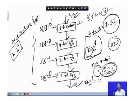
So, if I just added something like this if this is my x. So, this is my x, this is let us say S 3, this is S 2, this is S 1, and this is S 0. So, this is let us consider 8 bit controlled shift, this is 4 bit controlled shift, this is 2 bit controlled shift, this is 1 bit control controlled shift.
