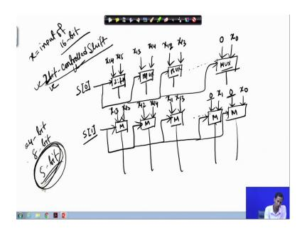
So, for this particular function for implementing what I require is that I require 1 bit controlled shift operation. So, 1 bit-controlled shift operation means what I need 2 is to 1 multiplexers. So, if I consider suppose this x input x is the input of 16 bit, let us consider that and I need 1 bit-controlled shift of that. So, at the time what will be, so, that means, here it will be up to x to the power 14 x to the power 15, x 15, x 13, x 14, x 12, x 13 here it will be 0 and it will be x 0, ok.
