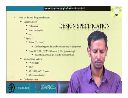
So, this design specification it starts with design specification. So, what are the main design considerations? whenever I am considering one design specification? So, at that time what do I consider in my specification? So, the first thing is that this design feasibility; design feasibility is basically that basically comes with this performance, power consumption and cost.
