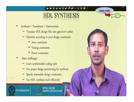
And then this once this functional simulation is done; then we have to follow this HDL synthesis. So, HDL synthesis means I have described it using language now I have to after that synthesis means what? It has to from the HDL coding it has to map to the corresponding using some of the logic gates so; that means, you just see that first thing this translate HDL design files into the gate level net list.
