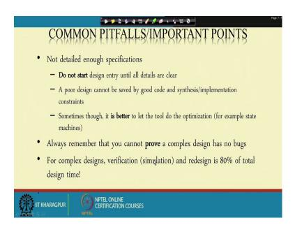
So, the common pit falls or the important points you have to be keep in mind that is, not detailed enough specification, do not start design entry until all details are clear, a poor design cannot be saved by good code and synthesis implementation constant. Sometimes tough it is better to let the tool to do the optimization; that means, it is not that the
