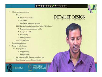
So, after that you have this detailed design, detailed design means you can you can chose in different two style that is in schematic or using HDL language any of these you can describe the corresponding; that means, once this architecture has been developed, then using this using any of this two schematic or HDL language HDL in language entry, any of this style you can chose for describing that particular architecture into the corresponding hardware.
