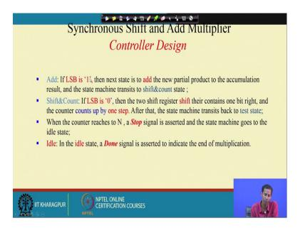
So, if LSB is 1, then next state is to add the new partial product to the accumulation results and the state machine transits to shift and count state ok. That means, what I said that whenever; that means, this LSB of this is 1. So, at the time what I have to do? I have to do this addition operation and shift and count; that means, this shift and count also I have to perform right.
