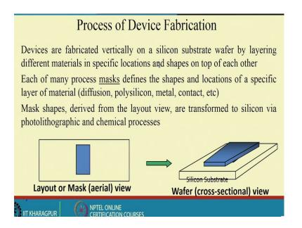
So; that means, this is the process of device fabrication I will not go details about this; that means, one thing this geometrical; that means, files you has to be sent to the fabrication. So, then this fabricating lab or this fabrication lab they have to follows through the device fabrication procedure and they after that, they build the corresponding system for me.
