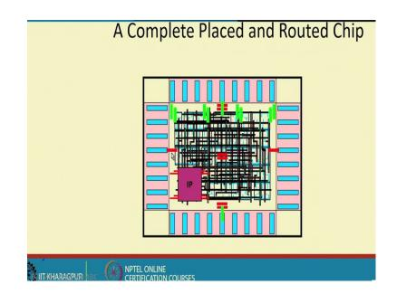
So, this is just one example of one complete placed and routed chip under the; that means, if I follow this ASIC designs style.
