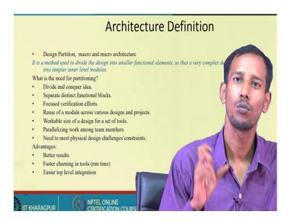
So, this architecture definition so we are this course is all about this architectural designs of ICs first the thing is that architecture definition. So, what does it means ok. So, this you have to build one system so at that time the design will be for a larger design it has to be partition into two, into two architecture you can just partition it, one macro architecture and another is the micro architecture.
