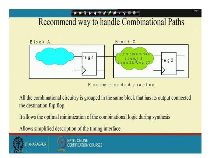
So, if you just see another logic; that means, the two things two registers it has. So, combine all the logic 1, logic 2, logic 3 level into one system and you this is the block A and this is the block B. So, here you see this is block A, this is block B and then block C, instead of that you just put it, this one as a block A and this one as block B or block C.
