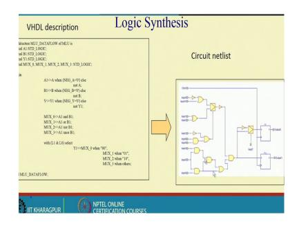
So, this logic synthesis is that here is this VHDL code which I have; that means, this is the logical expression which I have written using VHDL language and this is the corresponding gate level net list or the circuit level implementation of the corresponding circuit, what I have described using VHDL.
