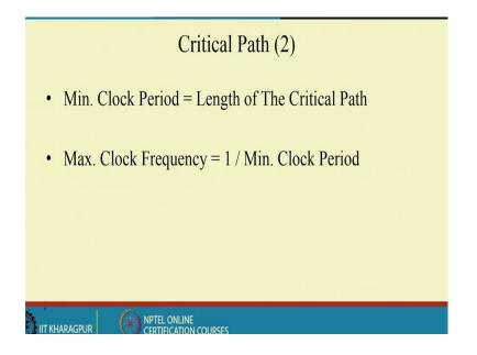
We will come to the later slide. So, once you got the critical path, so the maximum minimum clock period is the length of the critical path and then the maximum achievable clock frequency equals to 1 by this minimum clock period. So, this is the definition of maximum clock frequency and this is the definition of the critical path.
