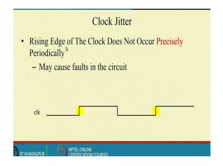
So, then another information; that means, another important part of this is the clock jitter. So, it happens that we consider or we for a synchronous design we consider that each of the system will be work on a particular age of the clock. So, it is not on not that only rising edge or the falling edge also, but it will it has to occur sorry it has to work on the edge of the clock, ok.
