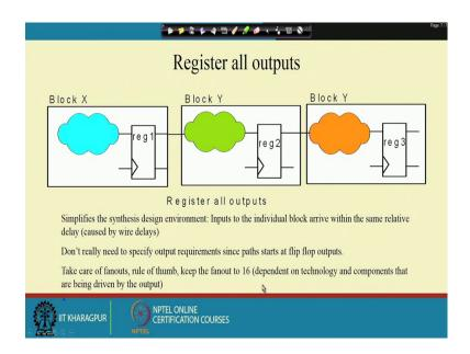
So, or else what you can do; that means, if I am having this kind of; that means, combinational logic. So, then I can put the registers here, after each of the combinational logic I can put the registers and so; that means, what does it means or this will basically avoid the, the problems which occurs during the synthesis, automated synthesis ok.
