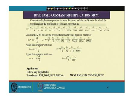
So, suppose in a constant multiplication operation ok, we are having this input and the coefficient. So, input and the coefficient means x in is the input and coefficient is nothing, but this a b and c. So, each of this if I consider each of these are of 16 bit, ok. So, 16 bit means if these input is x 1 ok, they are of 16 bit and this y 1, y 1 is basically a into x 1, ok that means what this y 1 is basically a into x 1, equals to y 1.
