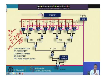
So, this is basically this for this x 1 plus x, x 1 plus x 1 by 2 that has been generated through this partial product unit and based on that in each of this additional operation is basically doing this.
