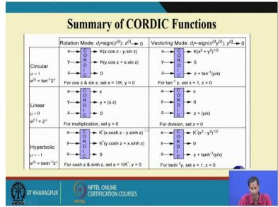
So, based on that so, we are getting three different equation and again this rotation vector whatever consideration we are taking for the rotation vector rotation mode and the vectoring mode, that will remain same; that means, the corresponding sign of d i that will be depended on this z for the that that rotation mode and for x i y i for the vectoring mode so, that will remain same.
