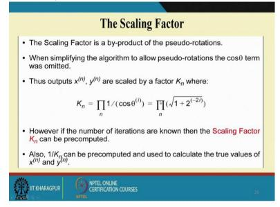
So, the scaling factor is a by-product of the pseudo rotation. So, what I said and we have already seen that because of the pseudo rotation from the original circular rotation as this the corresponding vectors that has been increased or; that means, magnitude of the vectors that has been increased. And when simplifying the algorithm to alive the pseudo rotation in the cos theta term was omitted that also we have seen.
