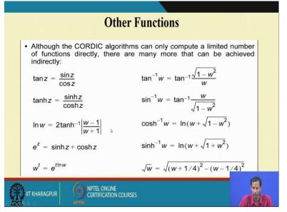
So, then again you can although this cordic algorithm can compute a limited number of function directly, but there are many more other can be achieved indirectly. So, tan z can be calculated divided using this sin z by cos z; then tan hyperbolic z you can calculate using sin hyperbolic z by cos hyperbolic z means what; cordic you run for to calculate this sin and cos, you run that for circular mode circular in the circular; that means, this circular rotation mode you are getting sin and cos.
