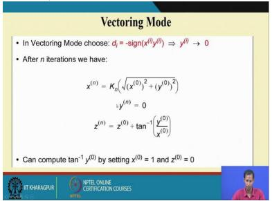
So, what we have to do? Actually this is whatever we are doing considering this fact, this is basically rotational mode I am doing or this mode is basically known as rotation mode. Now I can run this in the vectoring mode. The same algorithm I can just change it in a different form. So, that it will be run on the or it can calculate or it can compute different function, where the mode is basically known as vectoring mode.
