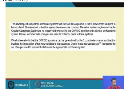
So, the advantage of using this other coordinate system with the cordic algorithm is that it allows more function to be calculated, but the drawback is that the systems became
