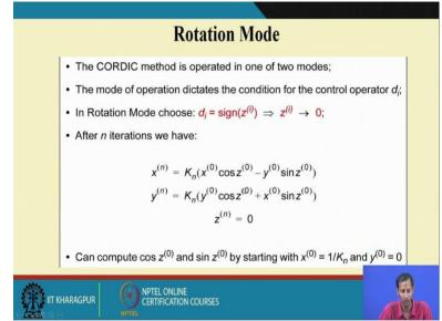
So, now considering this fact we can basically run the cordic in the 2 mode ok. So, one of the 2 modes we can run so, this is the basic equation.
