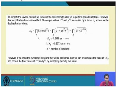
So, now if I say that to simplify the given rotation we remove the cos theta terms to allow us to perform the pseudo rotation; however, this simplification has a side effect and thus the output values of x n and y n scaled by the factor put the same logic whatever I am telling you. And the; that means, if I considered that n ok; that means, up to infinity the values will be K n values will be 1.6476. So, 1 by K n equals to what? 0.6073 ok.
