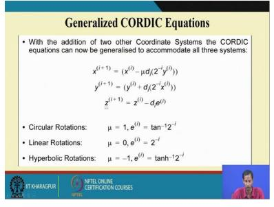
So, we will see that shortly. So, that if we consider this particular equation as the base equation. So, circular in the circular; that means, here what we have considered that another term over here which is mu. So, mu is basically changed for the circular rotation mu is 1 means this equation remains same and e i equals to tan inverse of 2 to the power i; the pseudo rotation becomes tan inverse of 2 to the power i.
