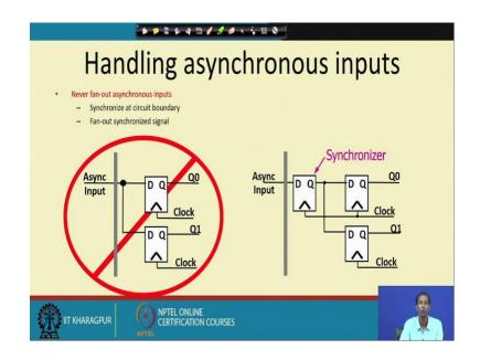
So, suppose I am having 1 asynchronous circuit something like this ok. Now asynchronous circuits asynchronous input like this means if I just connected it two different D flip flop which is clock at different end. So, at the time asynchronous input means it is coming at different time. So; that means, at the time it will reach to D 1 at
