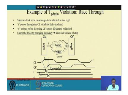
So, though because of this skew I we can get at sometime we can get this kind of thing ok. So, then again another example of this T pd minimum violation, which is the race through. Suppose the same kind of structure if you just see and here because of this clock skew, because of this clock skew the data changing at i that can happen early.
