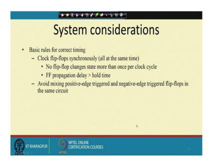
So, keeping that thing in mind we do this timing analysis right. So, again today we will see that, some of the things which are not yet covered in the timing analysis. So, that how we can; that means correct the timing correct the timing means: suppose. Actually till now we have discussed suppose the skew which is for a synchronous design.
