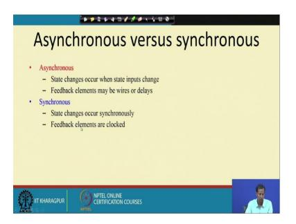
So, then what is synchronous design and what is asynchronous design? In synchronous circuits, the state changes occur when state inputs changes. The feedback elements maybe wires or delays in asynchronous circuits, but in synchronous circuits the state changes occur synchronously feedback elements are all clocked ok.
