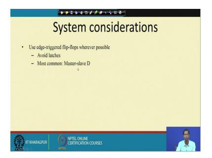
So, then use of this edge triggered flip flops instead of latches, why; because latches level sensitive not egde sensitive ok. So level sensitive means, it is not that it depends on the only on the clock and then; that means, the highest priority at that particular circuit is clock.
