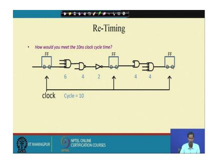
Now, another thing suppose here we are having 1 circuit right. So it says that, how would you meet the 10 nanoseconds clock cycle time for this particular path? That means, when these clock cycle will be 10 nanoseconds.
