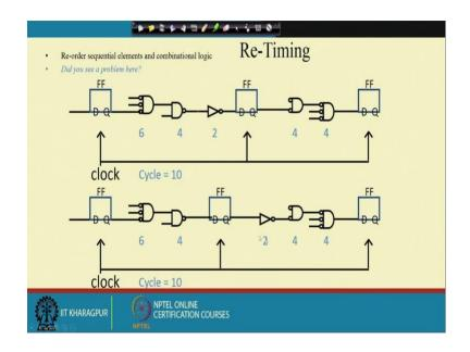
So, at the time what I have to do? I have to do a technique which is; that means, named as this re timing. So, what we see that here in this path it is taking 6 plus 4 plus 2; that means, 12 over here and in this it is having 4 plus 4.
