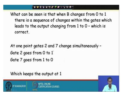
So, if you just see what can be seen is that when B changes from 0 to 1 there is a sequence, there is a sequence of changes within the gates which leads to the output changing from 1 to 0 which is correct. At one point gates 2 and 7 changes simultaneously; that means, gate 2 changes from 0 to 1 and gate 7 changes from 1 to 0, which keeps the output at 1.
