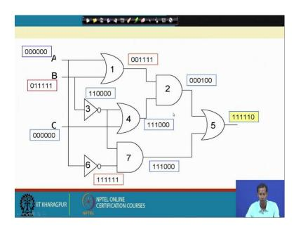
That means all to A C to 0 and B changes, initially A B C all are 0 and then this B changes to logic 1 what will happen. So, initially this all is 0. So, all this 0 means OR is 0; so, this is 1, this is 1 then after that what is happening? So, 1 and then 0, this is 1, this
