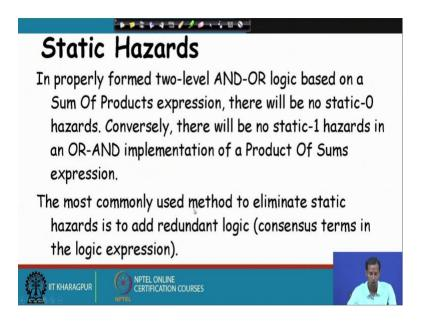
So, the static hazards mostly it is formed in two level AND-OR logic based on a Sum of Products expression and there will be no static 0 hazards. Conversely, there will be no static 1 hazards in an OR-AND implementation of a Product of Sum expression. The most commonly used method to eliminate the static hazard is to add redundant logic. So, how to add redundant logic, that also we will see.
