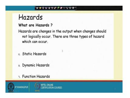
So, the first thing is that what is hazards? Hazards are changes in the output when changes should not logically occur, means this is unwanted changes. So, there are three type of that means, hazards are present which is the first one is static hazard, then dynamic hazard, then function hazards. So, what are these hazards? When this is occurring and how we can remove we will see in today's lecture. So, first we will talk about what is static hazards.
