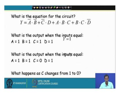
Now, suppose if I take the corresponding example of this so, at the time we can visualize the corresponding logic 1 hazard at the output which is Y. So, let us start with that. So, this suppose consider one equation where is Y equals to A bar and B bar C bar and with D and A B C and then B C D bar.
