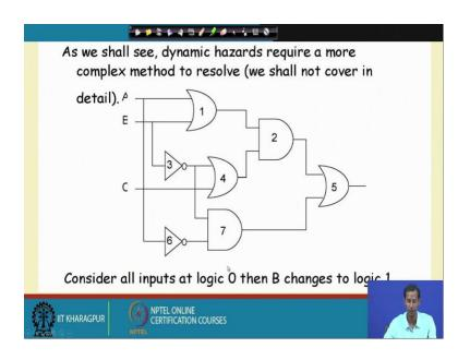
So, then if we take the example of dynamic hazard then you see suppose this is the; that means, there is several paths which are basically going from input to the output. So, here you see now as we shall see dynamic hazard requires a more complex method to resolves. So, consider all inputs at logic 0 then B changes to logic 1.
