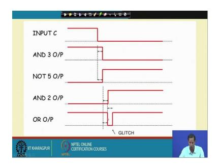
If you just see, suppose if I consider the corresponding changes in this. So, input C is changing input C is basically at 1. So, then AND 3 output means this is the AND 3 output. C is 1 A B D all are 1 right so, A B D all are 1 means C is 1. So, in AND gate what happens? If the other input is 1 then it depends upon the corresponding value of the other input. Here, if you see this is the AND output, this is the third gate or I have just numbered it as 3.
