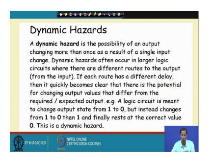
So, then you this is the; that means, in static hazard we are we can have two hazards: one is static; that means, this static 1 and another one is static 0. Then dynamic hazard, what is dynamic hazard? Dynamic hazard is the possibility of an output changing more than once as a result of a single input change. Dynamic hazard often occur in larger circuit where there are different routes to the outputs.
