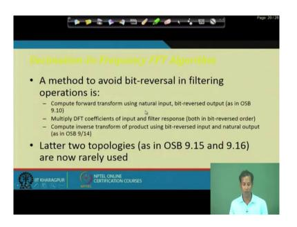
So, the decimation in frequency FFT algorithm it has to; actually this is a method to avoid; that means, what method we will adopt to avoid these bit reversal in filtering operation is to compute the forward transform using natural input and bit reverse output. And these multiply these DFT coefficients of input and filter response. Compute these inverse transform of the product using bit reversed input and the natural output.
