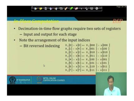
So, in decimation in time flow graphs require two sets of registers one for the input and other for the output for each stage. And note the arrangement of the input indices are in bit reversed in indexing.
