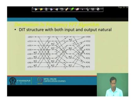
So, in decimation in frequency case so that the initial computation will be  $x \ 0$  with  $x \ 4$  then  $x \ 1$  with  $x \ 5 \ x \ 2$  with  $x \ 6 \ x \ 3$  with  $x \ 7$  and then we will get the corresponding output something like this.
