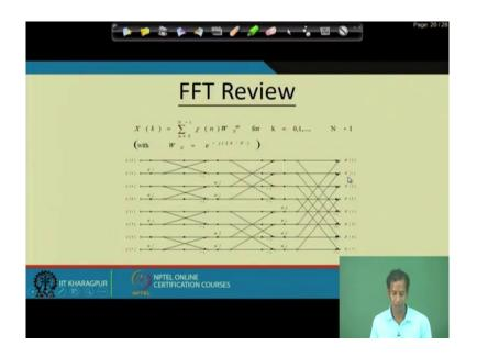
So, this is the; that means, this decimation in time fast Fourier transform architecture. Now, actually whenever we have to design these particular circuit so at the time the hardware implementation this is the just that the flow of; that means, how this data flow diagram of this fast Fourier transform. Now these I have to convert or this I have to this data flow diagram will be implemented via some hardware.
