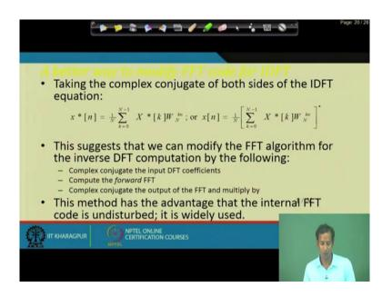
So, what will happen if we design the I FFT block? So, at that time how we can do; that means, how we can modify the FFT code so that it becomes the inverse; that means, inverse fast Fourier transform ok. So, what we can do is that at that time it will be just 1 by N into k; that means, k 0 to N minus 1 with x convolution with these W N into N base k n ok.
