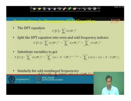
So, these decimation in; that means, FFT algorithm. So, this is the initial DFT equation. Now if we split this DFT equation into even and odd indices; that means, frequency indices then these particular equation can be written as n 0 to N by 2 minus 1 summation of these n 0 to N by 2 minus 1. Where x n into W N into n 2 to 2 r whereas, the; that means, this is the even part and this is the odd part; that means, the DFT now it has been split into two. So, that I can run parallelly ok.
