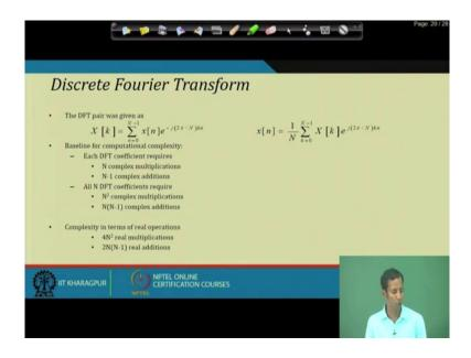
So, at the first actually we have to consider these Fourier transform which came for digital signal passing is these discrete Fourier transform. So, this is the; that means, equation for these generic discrete Fourier transform.
