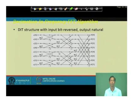
So, in decimation in time actually then this DITs; that means, decimation in time structure with the input bit reverse the output will be natural; that means, if we apply the input in a bit reverse manner which is these x 0 x 4 x 2 x 6 x 1 x 5 x 3 x 7 so at that time the output will be comes in the bit reverse manner.
