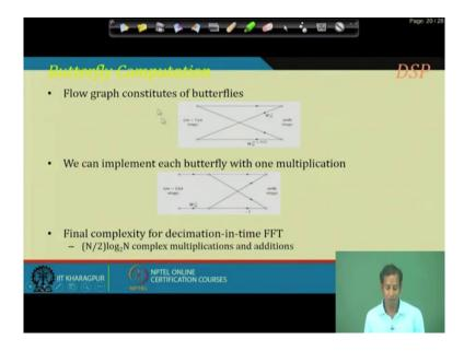
Now, what is these butterfly computation? So, the butterfly computation is that it actually generates from the m minus 1 stage, it has to multiply it with the corresponding twiddle factors to generate the next stage, which is the m th stage ok. So, in these upper ward actually this upward; that means, branching it has to multiplied with W dash W r N whereas, this lower branch has to multiply with the twiddle factor values of W N r plus N by 2.
