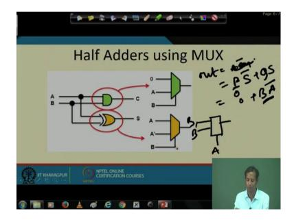
Now, we will see how to implement the half adders using multiplexers. So, according to the logic of half adder, what we need is that; we need to implement the carry we need one AND gate and to implement the sum we need one XOR gate.
