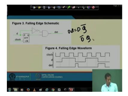
So, at that time, in falling edge what we have to do? In earlier case what was there the inverter was placed over here the data input was coming there, but here what I did, I just placed I just interchanged this position of in inverter in the upper path. So, at that time what will happen? At this particular edge; this negative edge it will give me one pulse and again at these particular edge it will give me another pulse.
