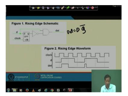
So, this is used for positive edge sorry, falling sorry, rising edge and for this what is this in this case this is D bar Q. So, when I need to combine both together in the particular circuits so, at that time so, at that time what I need? I just need to add them. So, if I add them DQ bar and D bar Q is nothing but D sorry D XOR Q. So, that has been done over
