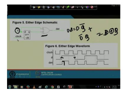
Now I need; that means, both the edge should be detected at the output ok. So, then how to do that? Then that can be done using if I use instead of this here what we are doing? Here we are we are doing if I say that this is what this is D into Q bar ok.
