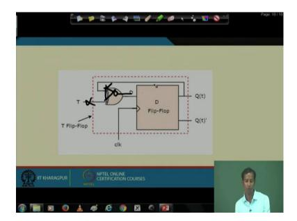
Now, then again if the question has been asked to make these as T flip flop. So, the D flip flop we already made ok. So, then again actually T flip flop means we have to the D flip flop, the output from the D flip flop that will be just inverted and it will go to the D input of the corresponding flip flop. So, D flip flop using this 2 is to 1 multiplexer we have already designed.
