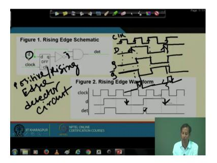
So, then we will see another example which is very basic circuit for this edge detector; that means, whenever, what is this edge detector? Whenever this clock edge occurs so, at that time it will detect that there is one edge of the clock which is happening. So, how to detects? Actually, there will be this rising edge, there will be falling edge of the clock and we can also detect that rising and falling both altogether.
