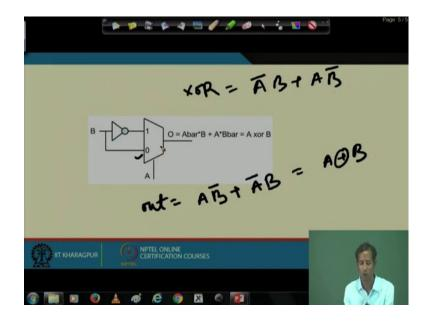
Now, let us consider another example ok. So, where I have to design these particular multiplexer should be work as a XOR gate ok. So, in XOR gate the corresponding logic for XOR gate is what? This XOR function says that it will be A bar B plus AB bar ok.
