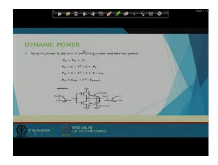
So, now we will see that the corresponding equation for dynamic power. So, as we have already discussed that dynamic power is the sum of the switching power and the internal power. So, if I just write that equation in the equation form if I just write, then P D the dynamic power consumption will be the PS is the switching power plus this PI is the internal power. So, the switching power I can write that is C V square f and the PI is V into I SC, I SC is the short circuit current.
