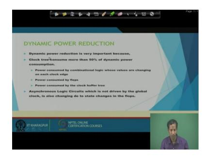
So, then dynamic power reduction. Dynamic power reduction is very much important because the clock tree path consumes more than 50 percent of dynamic power consumption. And, power consumption by combinational logic whose values are changing on each clock edge power consumed by flops power consumed by the clock buffer tree. Asynchronous logic circuit which is not driven by the global clock is also changing due to the state changes in the flops.
