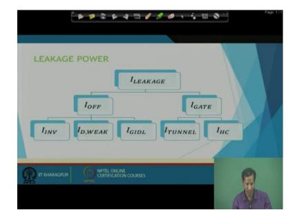
So, if I just actually make the chart so, then I leakage it is having I OFF plus I GATE ok. So, I OFF contributes is the summation of the contribution from I inverter reverse bias current ID weak that is the sub threshold drain current. And then, I GIDL GATE induced drain leakage current then the I GATE current is basically the tunneling current gate tunneling current and the hot carrier injection current.
