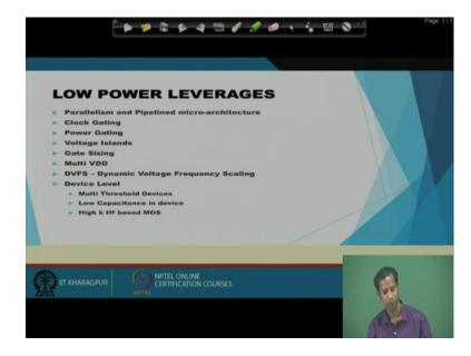
So, other actually the low power techniques there are several techniques to achieve this low power is that one of this; that means, major techniques we use is that parallelism and pipelined micro architecture. Then, there are clock gating options, there are power gating options, there are voltage islands, there are gate sizing, there are multi VDD approach, there are this DVFS Dynamic Voltage Frequency Scaling.
