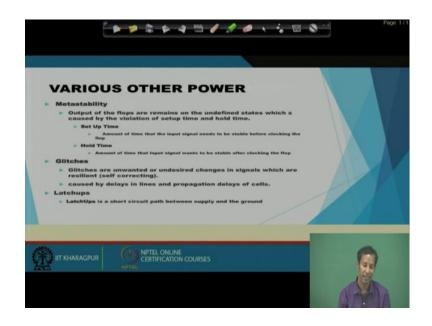
So, then there are other actually various power one of the power is that meta-stability. So, output of the flops remains on the undefined state, which is caused by the violation of setup and hold. So, we know what is the set up and hold and in digital systems, when we can get this meta-stable state, that also we have already seen ok. So that means, if we get 1 meta-stable state in in is digital circuit design so, at that time it can creates a lot of power consumption into the circuit.
